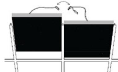
Connect a Jumper Cable to the first panel and connect it to the next panel. Up to 50 Kinetics Panels can be connected together in any configuration. If
