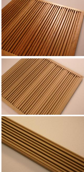
Using Manfred Schroeder's diffraction number theory, our new HighTones2 Diffuser design offers improved "equal energy" diffusion. This is accomplished via two design methods: a higher order well sequence, offering more available well depths for smoother diffusion; and Barker code implementation, offering reduced lobing that results from repeated sequencing (Fig. 2).
